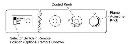
Figure 36 - Setting the Selector Switch, Control Knob, and Flame Adjustment Knob for Remote Operation
